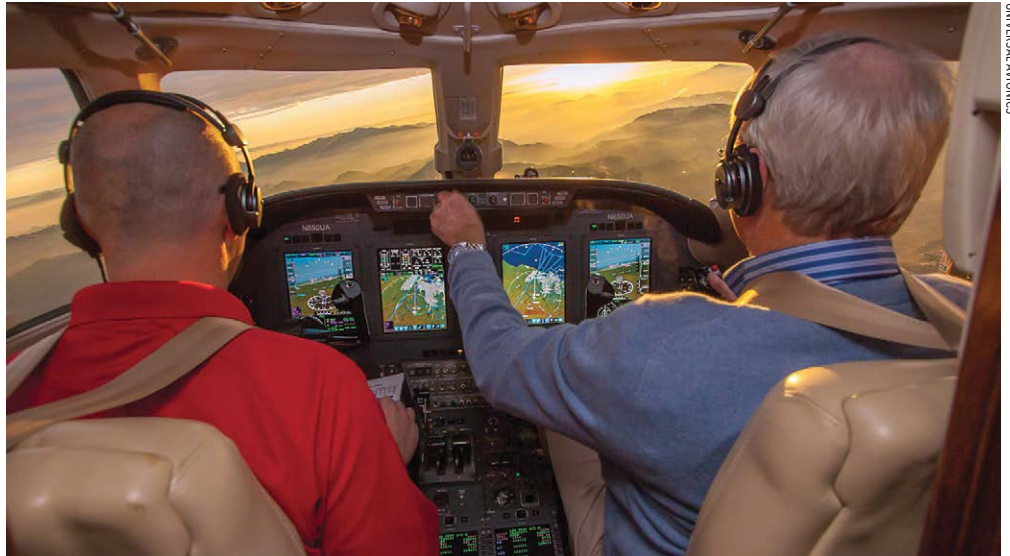
Universal Avionics’ InSight cockpit upgrade is shown undergoing flight testing.
