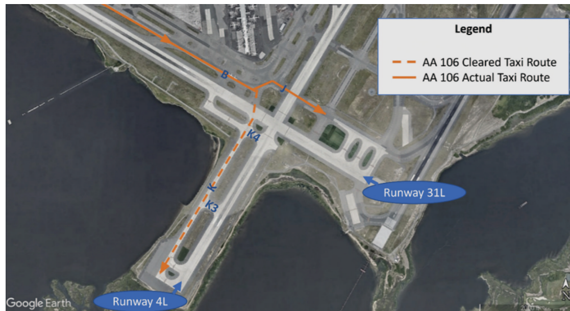
Depiction of American Airlines Boeing 777 cleared route versus the actual taxi route. Source: NTSB.
