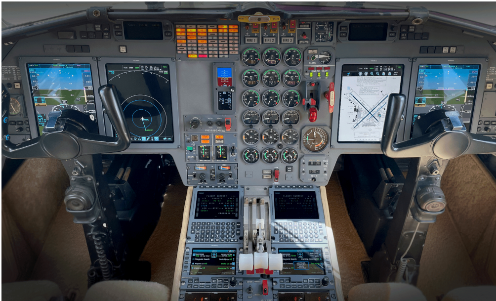
In 2022, Dassault obtained FAA supplemental type certificate approval allowing installation of the Universal Avionics InSight flight deck upgrade of the Falcon 900B. Universal Avionics
