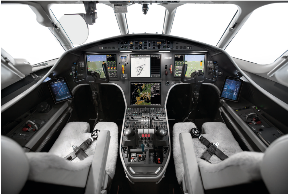
The Honeywell-based EASy II flight deck of the current-production Falcon 900LX. Credit: Dassault Falcon Jet
