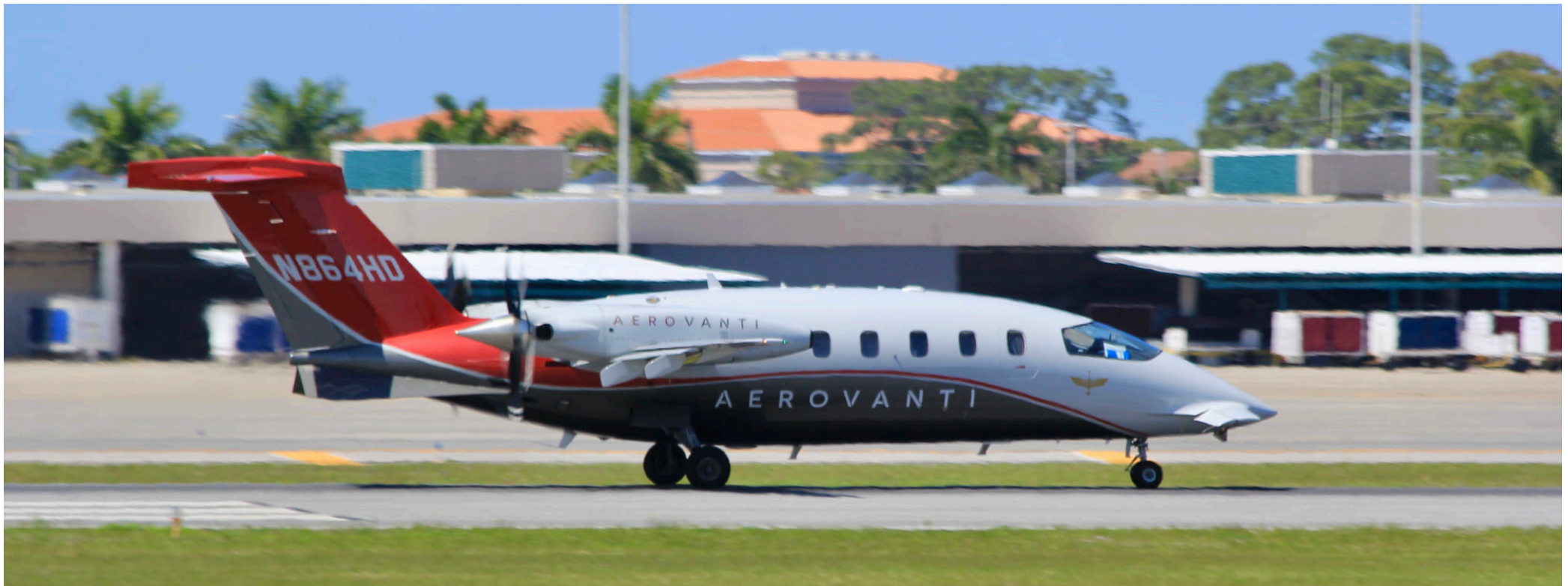
The Avanti was designed to match the speed of a jet with the fuel efficiency of a turboprop. Credit: Nigel Prevett/Aviation Week
