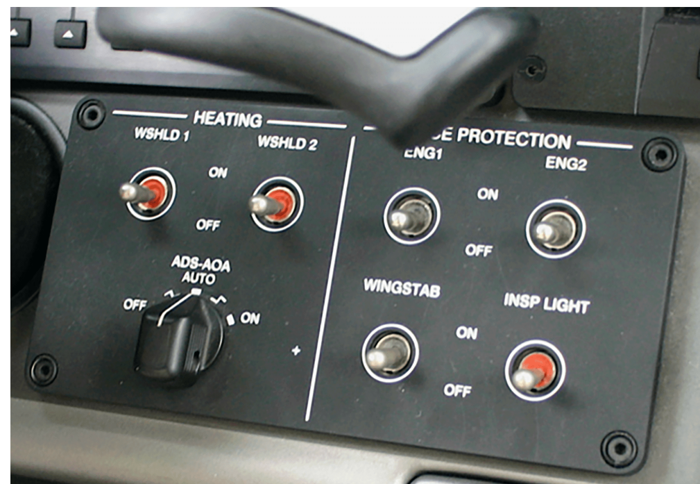
Phenom ice-protection panel. Credit BFU Germany
