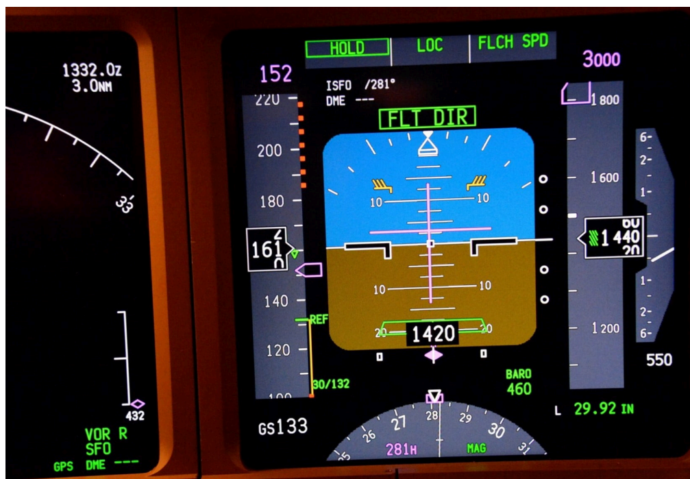
This shows how HOLD would be annunciated on the Flight Mode Annunciator. Credit: NTSB
