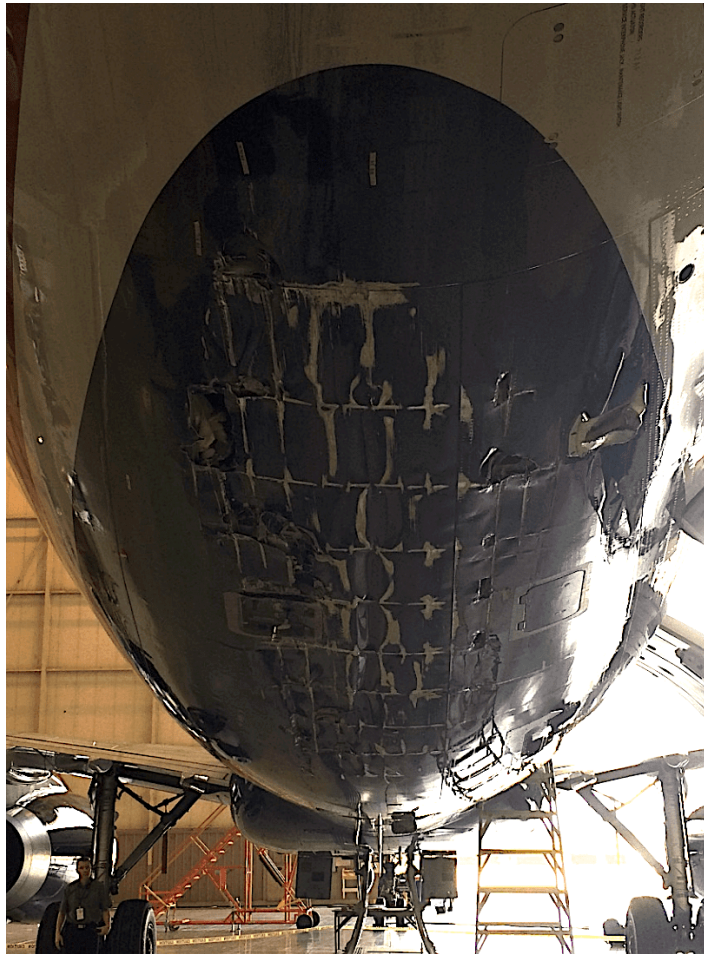
Damage from a tail strike is evident to the underside of this fuselage.
