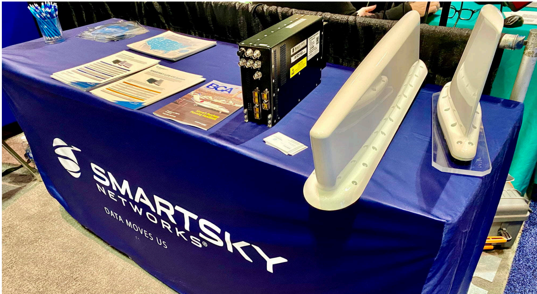
A SmartSky Networks shipset, including (l-r) an aircraft base radio, blade antenna and full-duplex quad antenna, was displayed during the NBAA Maintenance Conference in Hartford. Credit: Bill Carey
