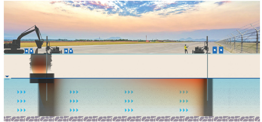
An injection rig introduces colloidal activated carbon in the subsurface to reduce PFAS to the non-detectable range in groundwater and eliminate PFAS risk caused by the AFFF release. Credit: Regenesis Concepts
