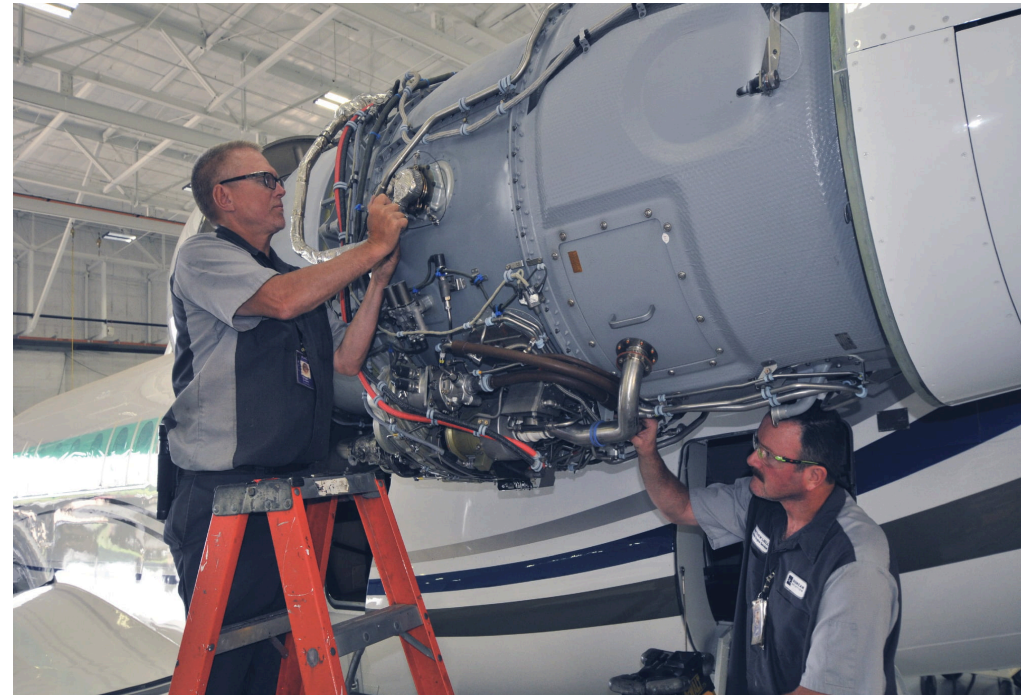
Duncan Aviation maintains a Pratt & Whitney PW308C on a Falcon 2000EX. Credit: Duncan Aviation
