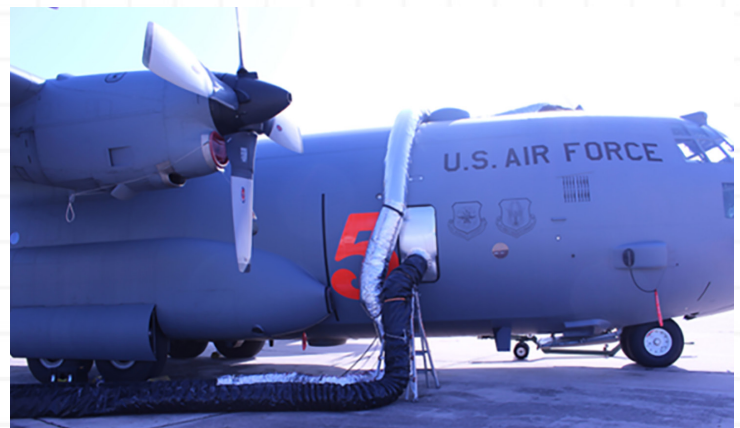
Decontamination using the Joint Biological Agent Decontamination System on a C-130 airplane interior is performed in July 2016 to extinguish mold. (Photos courtesy of Dr. Wendy Goodson, AFRL)
