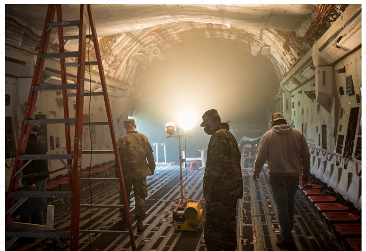
Air Force Research Laboratory team members look over a C-17 used to investigate the ability of ground heaters to raise interiors to temperatures sufficient to kill the COVID-19 virus. Photo Credit: U.S. Air Force photo/ Richard Eldridge
