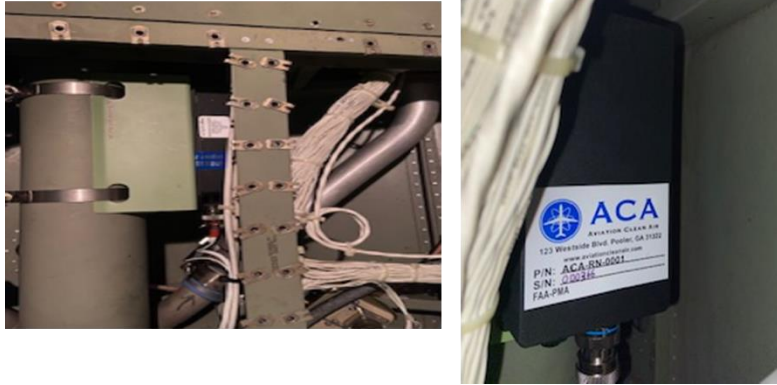
Figure 2: The ACA NPBI™ unit weighs less than one pound (right) and installs on the existing ECS output ductwork (left) to provide continuous protection from harmful pathogens.
