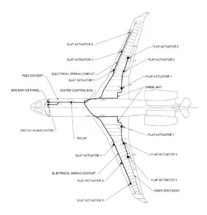
Wiring and component installation locations are described fully in the STC
