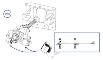
Wrap-around, cuff-style, design and are mounted on the exterior of the actuators
