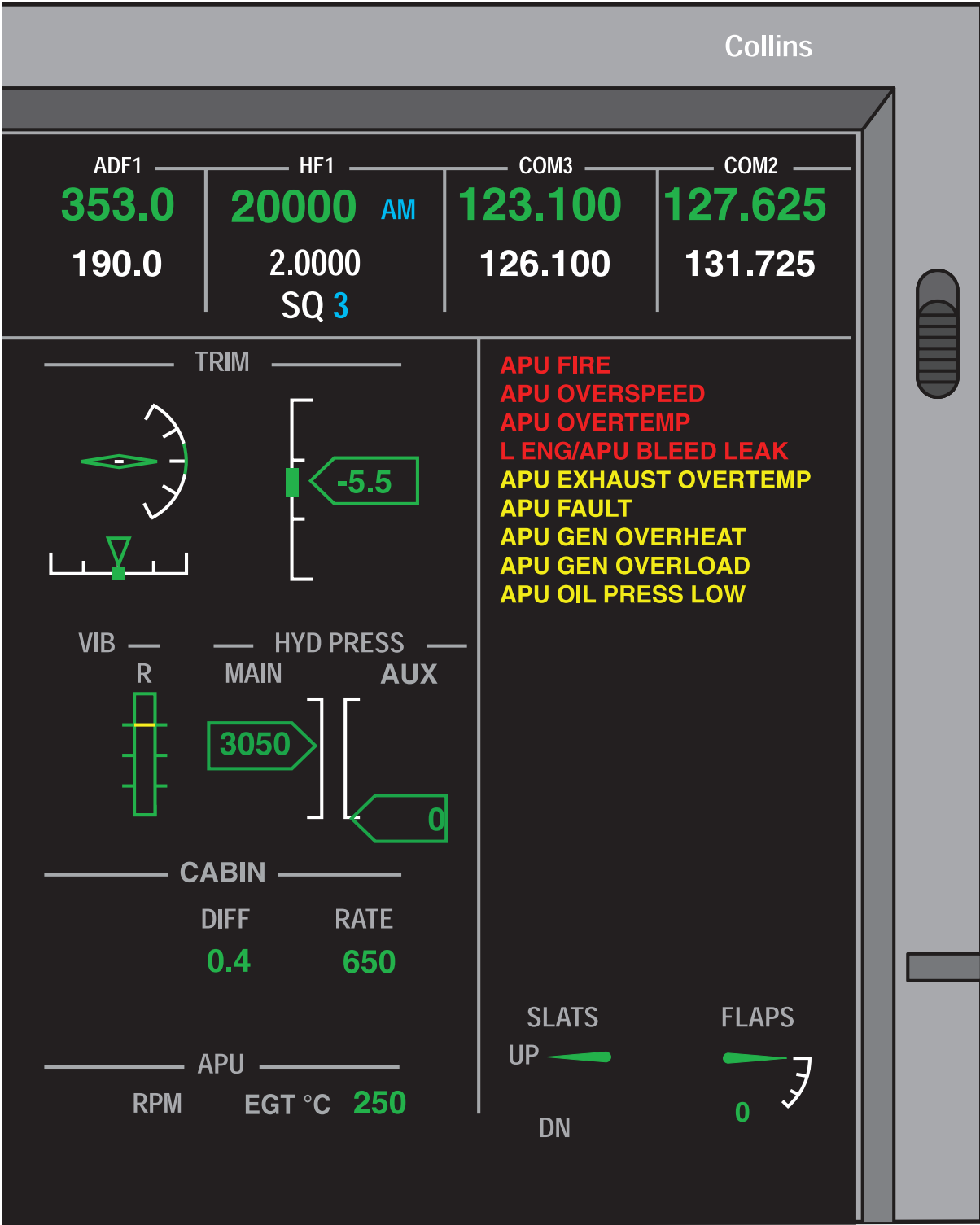
Figure 6-4. APU EICAS Indications
