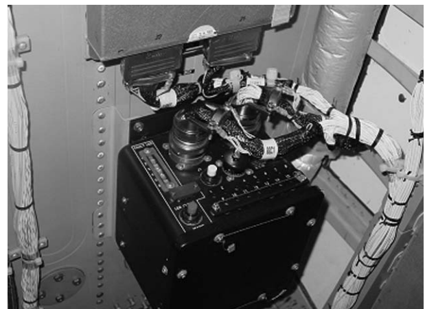
Figure 15-11. Flap/Slat Electronic Control Unit (FSECU)
