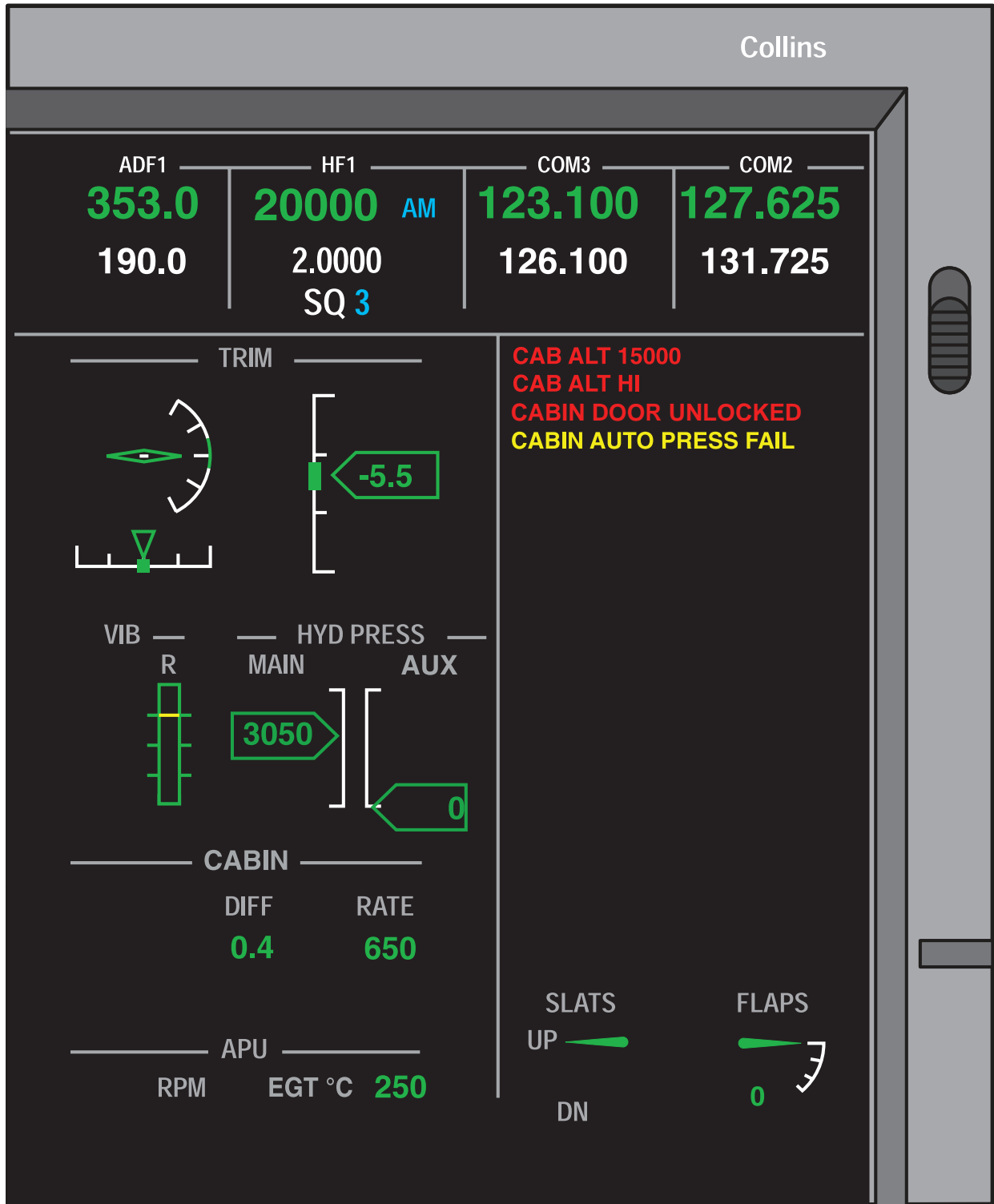
Figure 12-6. Pressurization System EICAS Indications
