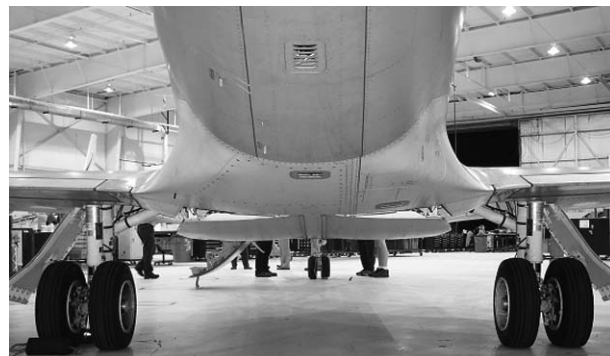
Figure 14-6. Main Gear Doors
