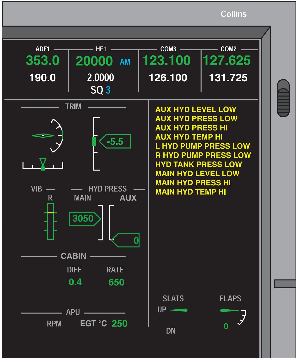
Figure 13-15. Hydraulic EICAS Indications
