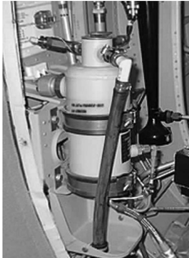
Figure 13-10. Auxiliary Hydraulic Reservoir
