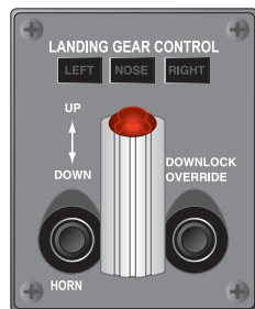
Figure 14-13. Gear Up and Locked
