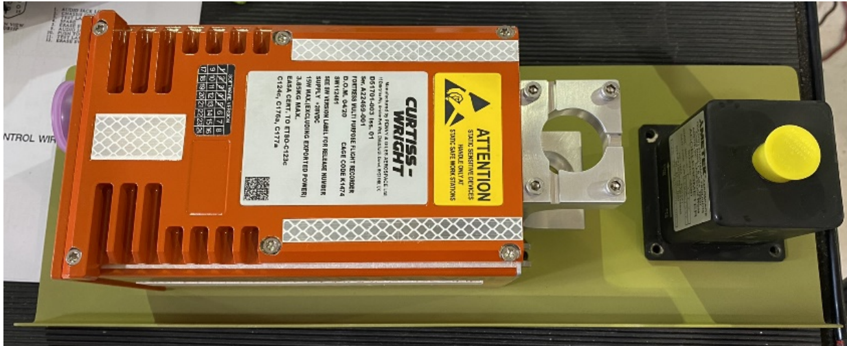
Figure 5: Recorder and Accelerometer Mounting
