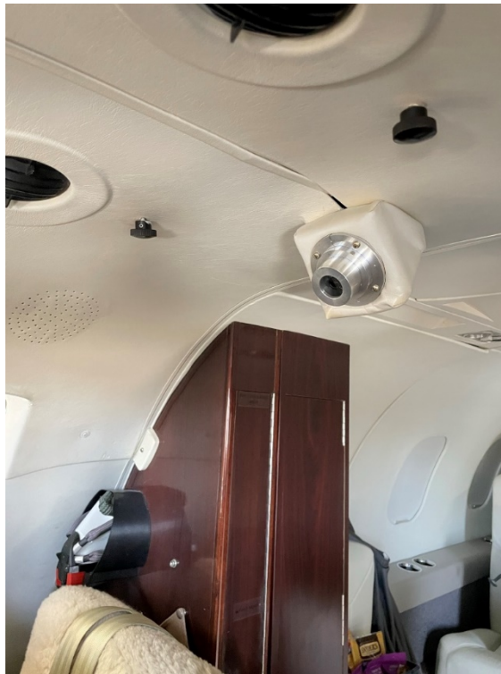
Figure 12: Typical Camera Installation
