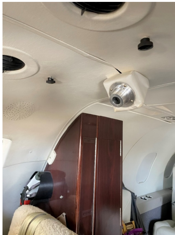
Figure 12: Typical Camera Installation
