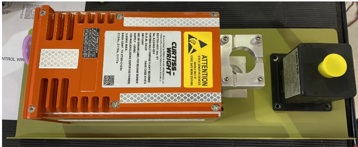
Figure 5: Recorder and Accelerometer Mounting
