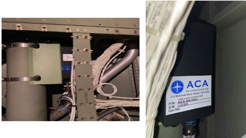
Figure 2: The ACA NPBI™ unit weighs less than one pound (right) and typically installs on the existing ECS output ductwork (left) to provide continuous protection from harmful pathogens.
