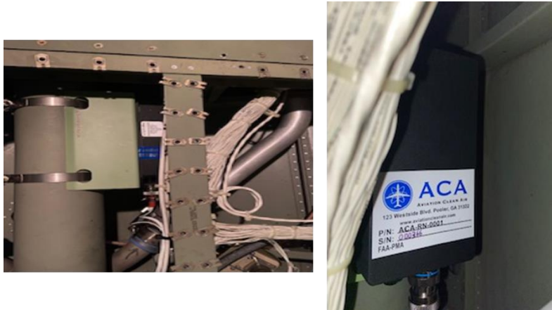
Figure 2: The ACA NPBI™ unit weighs less than 1.35 pounds/610 grams (right) and typically installs on the existing ECS output ductwork (left) to provide continuous protection from harmful pathogens.
