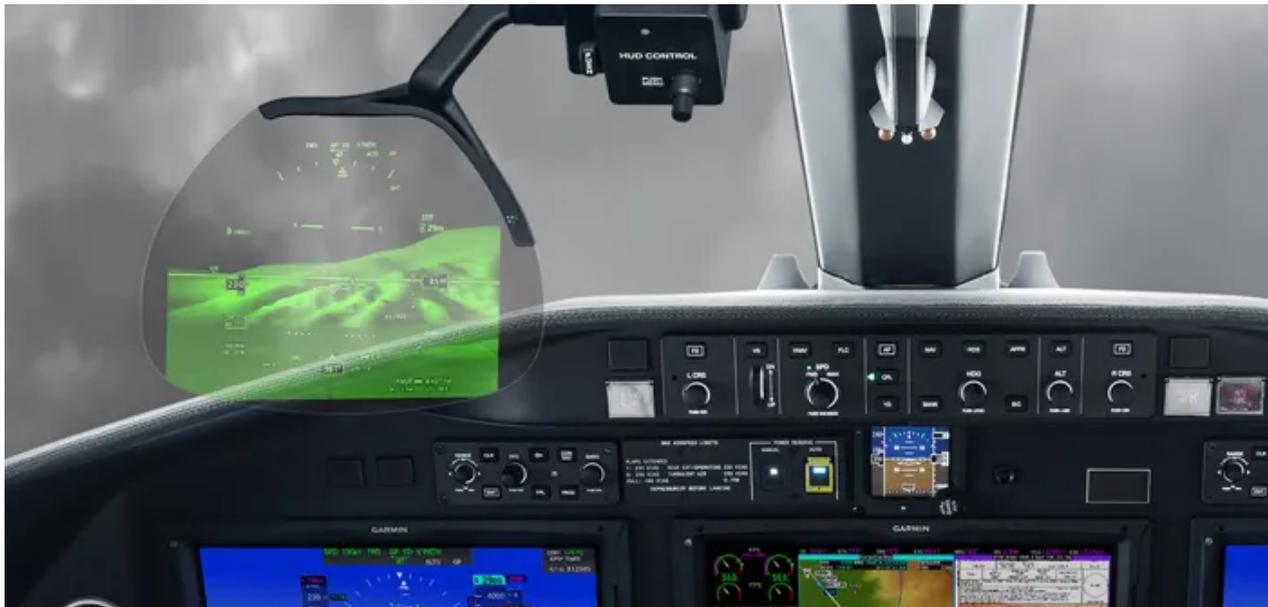
Designed to integrate seamlessly with our integrated flight deck systems for light- to super-midsize business aircraft, GHD 2100 HUD gives pilots a fully integrated “out-the-window” view of their primary flight display (PFD) information, overlaid with a synthetic vision virtual perspective. HUD technology allows pilots to fly more “eyes out” — and less “head down” — to maintain optimal situational awareness throughout every phase of flight.
